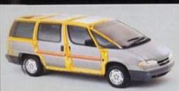
Steel Safety-Cage. The body's space frame is designed to surround passengers with a cage of steel. Structural steel beams inside the front doors and sliding side door are designed to help prevent intrusions into the passenger compartment during shallow-angle
