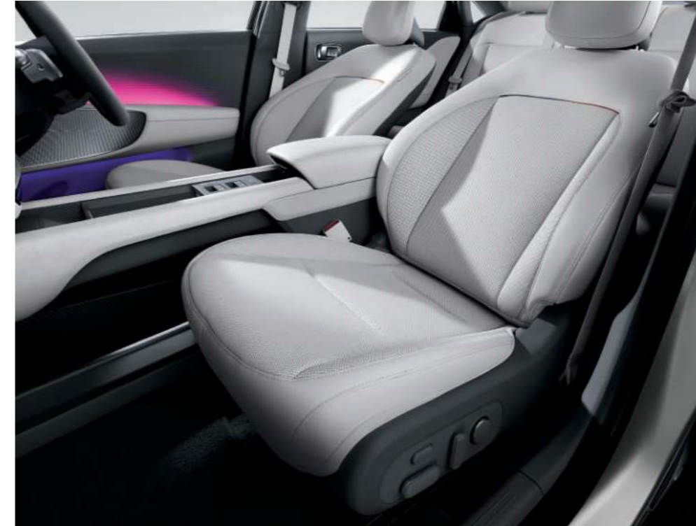
8-Way Powered with 2-Way Lumbar Support
