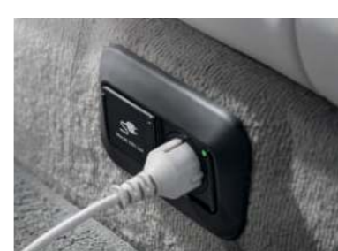
Vehicle-to-Load (V2L) technology
