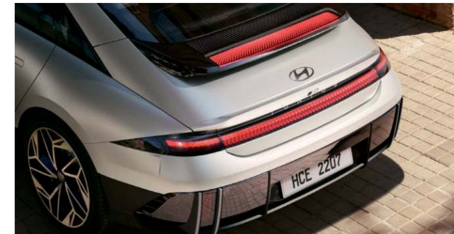
New Hyundai emblem Parametric pixel high-mounted stop lamp (HMSL) + Full LED rear combination lamps
