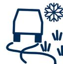
Grass/Gravel/Snow – maximises traction and control on firm, but slippery, surfaces. Wet leaves and grass or hard-packed snow and ice call for this setting.
