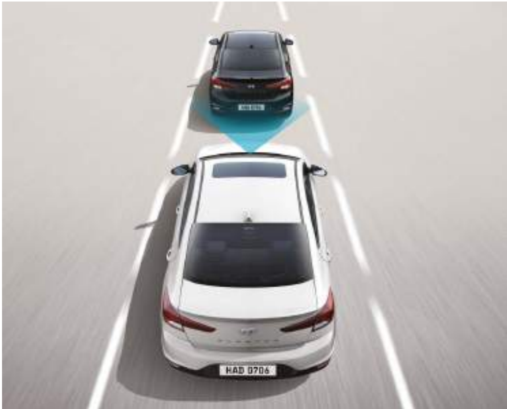
Forward Collision-Avoidance Assist (FCA) Front view camera is in place to warn the driver of imminent collisions with other vehicles; and if necessary, it applies emergency braking to mitigate from collision.
