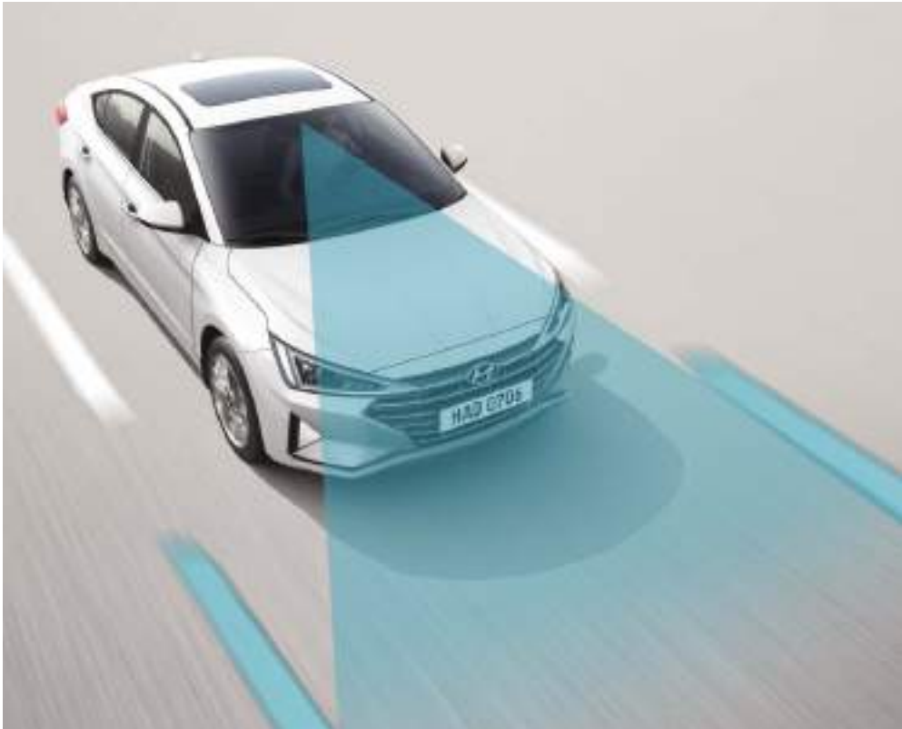
Lane Keeping Assist (LKA) Available in the Active Concept, a front view camera detects lane markers to prevent 'drifting' into lanes. In the event the vehicle strays from the lane, it prompts a visual and sound alarm, then automatic steering kicks in to keep it straight on its course.
